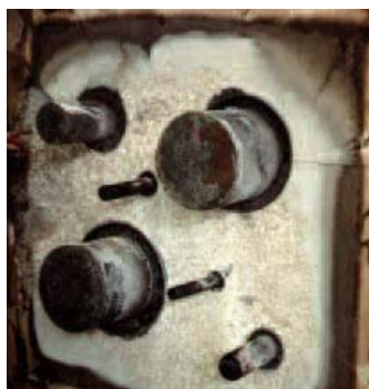
Test slab after hose stream. Cold water striking the 1900°F slab caused scalling of concrete, but left Link-Seal® modular seal intact. Unexposed side showed no evidence of water damage.
